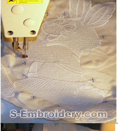
15. Place the hoop back on your machine and stitch out part #5. In the process of stitching part #5 will be integrated with parts of the design you created earlier. The stitching of part #5 will finish with stitching out the next set of alignment markers you will need for matching part #6 to the rest of the design.
