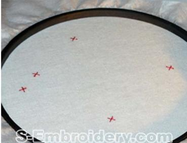
13. Hoop stabilizer for stitching part # 5 and do the alignment marks. Then take the hoop off the machine and place it on the cork tile.
